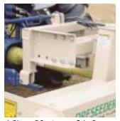
**Adjustable 3-way hitch** Exclusive versatile hitch design puts the Preseeder tiller closer to any make of tractor for better balance, control, and safety.
