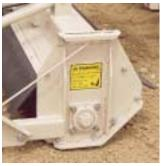
**Replaceable skid shoes**The skid shoes take a lot of abrasive wear and tear. That's why we make them from hardened steel. Models 605, 725 and 805 feature bolt-on replacements.
